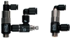
Piloted non-return valves are designed to protect installations: if the compressed air supply is removed, they lock the air supply to the cylinder, thus maintaining it in position.
