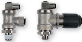
When the pilot signal is removed, these fittings ensure the safety of operators and protect the installation by cutting off the supply of compressed air in the circuit.
