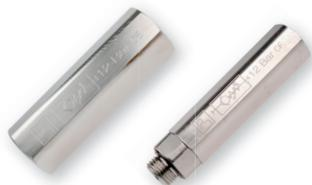
These nickel-plated brass adjustable non-return valves allow compressed air to flow in one direction and prevent flow in the other. They incorporate precise adjustment of opening pressure in the return direction.
