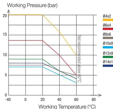
To calculate burst pressure, the values in these graphs should be multiplied by 3.
