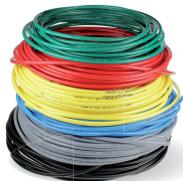
The PU tubing is available in 3 grades of ether, ester and crystal ether. Flexible with a small bend radius, it saves 50% of space for networks, compared to the semi-rigid PA.
