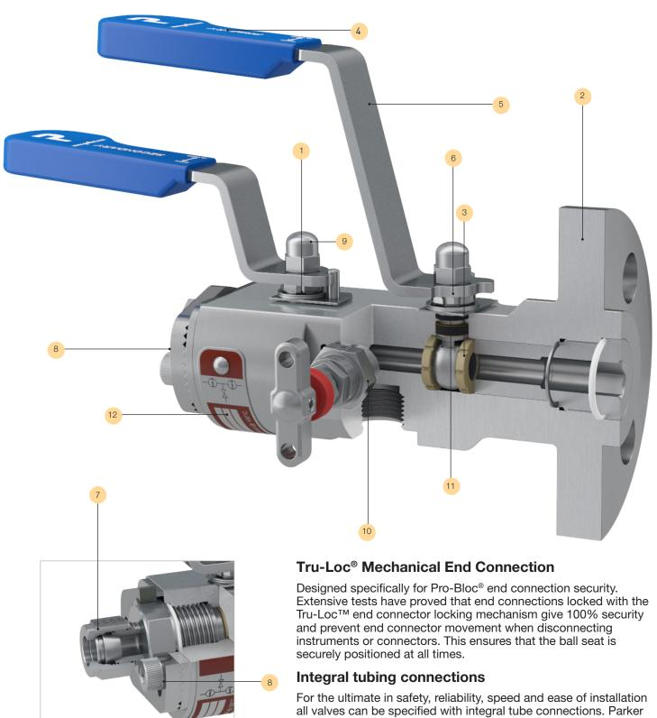
For the ultimate in safety, reliability, speed and ease of installation all valves can be specified with integral tube connections. Parker A-LOK® (Two Ferrule) or CPI™ (Single Ferrule) compression fitting technology.
