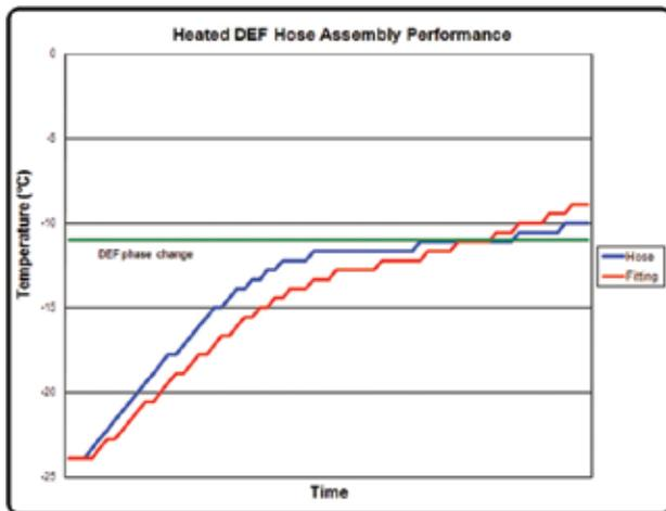
The thaw performance of a heated DEF assembly. The thaw performance and final hose assembly lengths are limited only by the maximum available power of the dosing system, Parker said.
