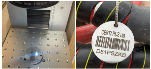
Certarus uses laser engravers to etch the PTS ID and barcode onto durable metal tags.
