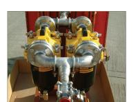
bolts. The slotted "locking ring collar" allows maintenance personnel to hand loosen the four collar bolts, rotate, and lower the bowl assembly for filter changeouts.
