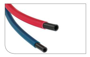
pressure air and water supply lines where weld spatter protection is required. The double wall design has a flame resistant jacket made from material that meets the UL94 V-0 standard. The specially formulated jacket material is easy to skive back, exposing the core tube for quick insertion into Parker's Prestolok PLM fittings.
