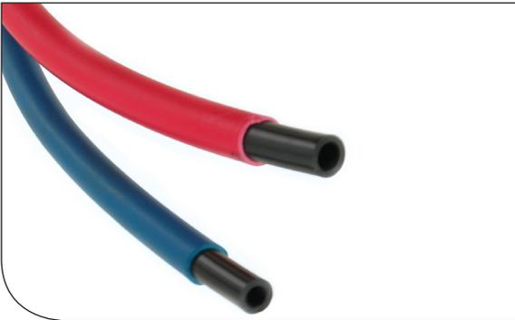
Parflex 95FR MicroWeld™ Tubing is an ideal option for low to medium pressure air and water supply lines where weld spatter protection is required. The double wall design has a flame resistant jacket made from material that meets the UL94 V-0 standard. The specially formulated jacket material is easy to skive back, exposing the core tube for quick insertion into Parker’s Prestolok PLM fittings.
