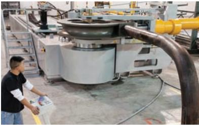
With state-of-the-art CNC large- and small-capacity bending equipment, as well as all complementary pipe end finishing equipment, the CPS team expertly manufactures *prefabricated piping assemblies*.
