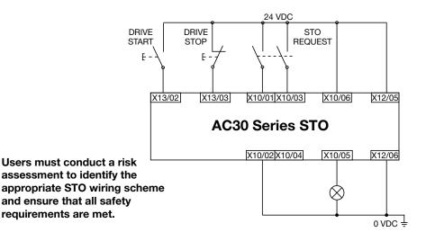
It is the user's responsibility to ensure the safe and correct use of the STO function of the AC30 Series. User's should read and fully understand chapter 6 (Safe Torque Off) of the product user manual. Manual No. HA501718U001
